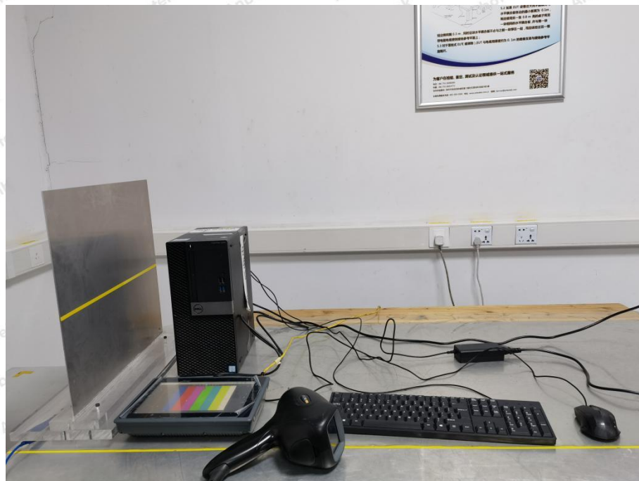
Photo of Electrostatic Discharge Immunity Test
