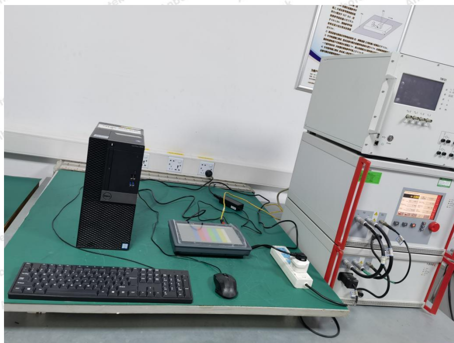
Photo of Electrical Fast Transient/Burst Immunity Test
