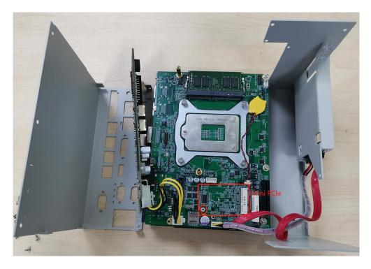
Picture 2.33: Mini PCle installation (1)
