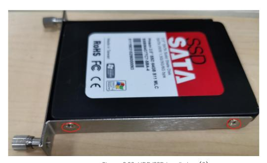
Picture 2.23: HDD/SSD installation (3)
