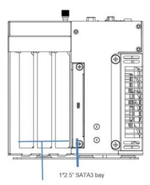
Easy disassembly Expansion Module 1\*PCle X4 slot, 2\*32bit-PCI slot
