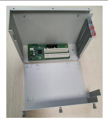
Picture 2.35: PCI installation (2)
