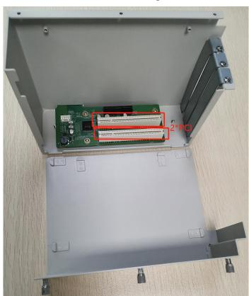
Picture 2.36: PCI installation (3)
