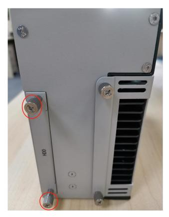
Picture 2.24: HDD/SSD installation (4)
