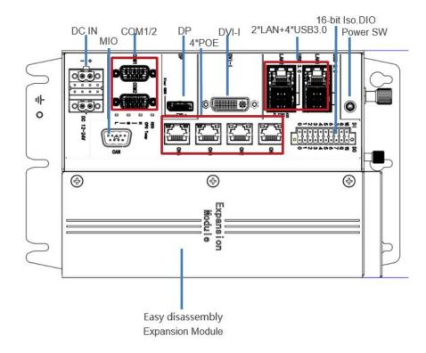
Picture 1.4: KGEC-6301-T001 Front Panel
