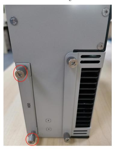
Picture 2.21: HDD/SSD installation (1)
