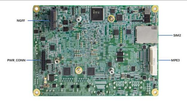
Figure 2.2 Jumper and Connector Location
