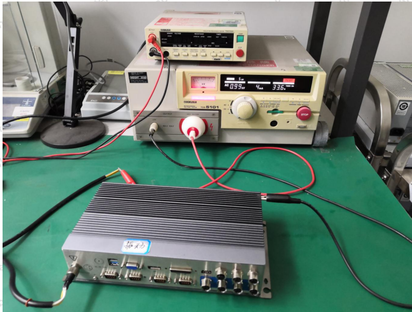
Voltage withstand test
