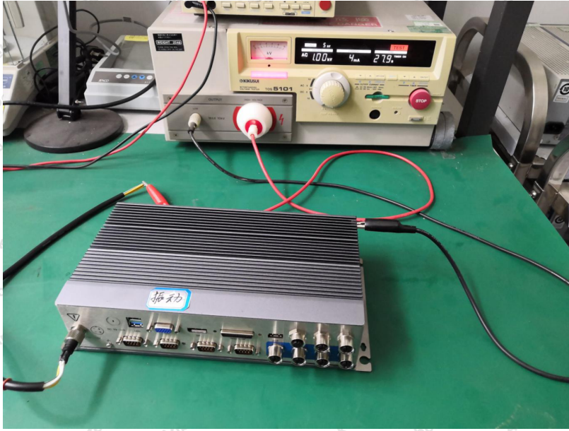
Voltage withstand test
