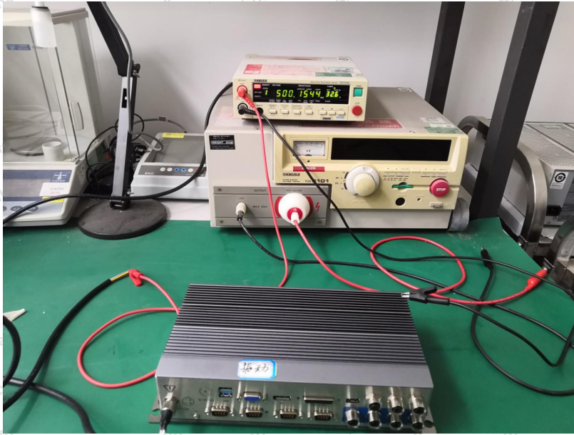
Insulation resistance test
