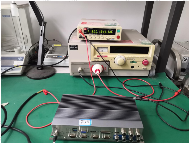
Insulation resistance test
