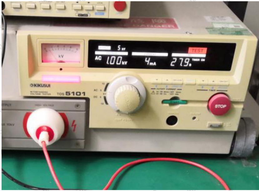
Voltage withstand test
