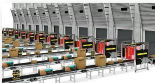
Logistics visual inspection
