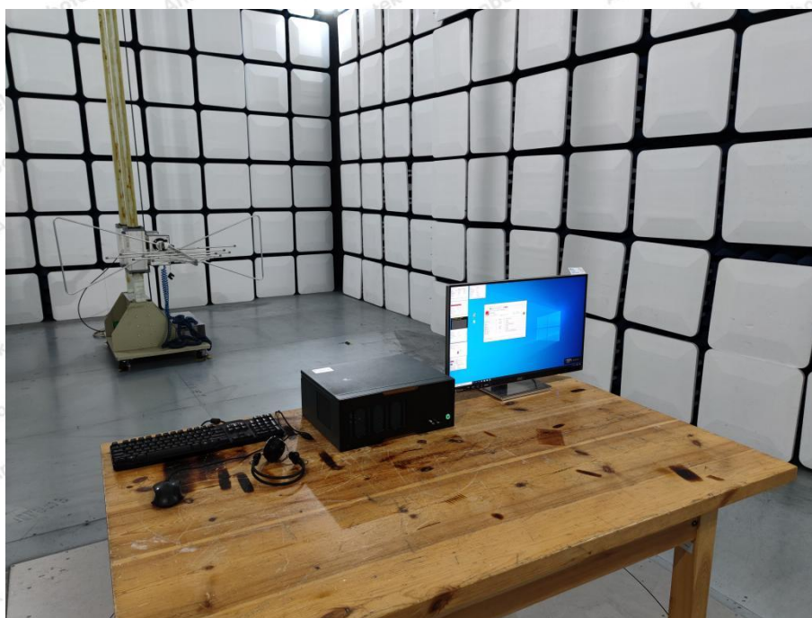
Photo of Radiated Emission Test
