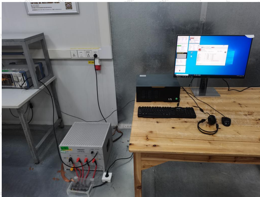
Photo of Power Line Conducted Emission Test
